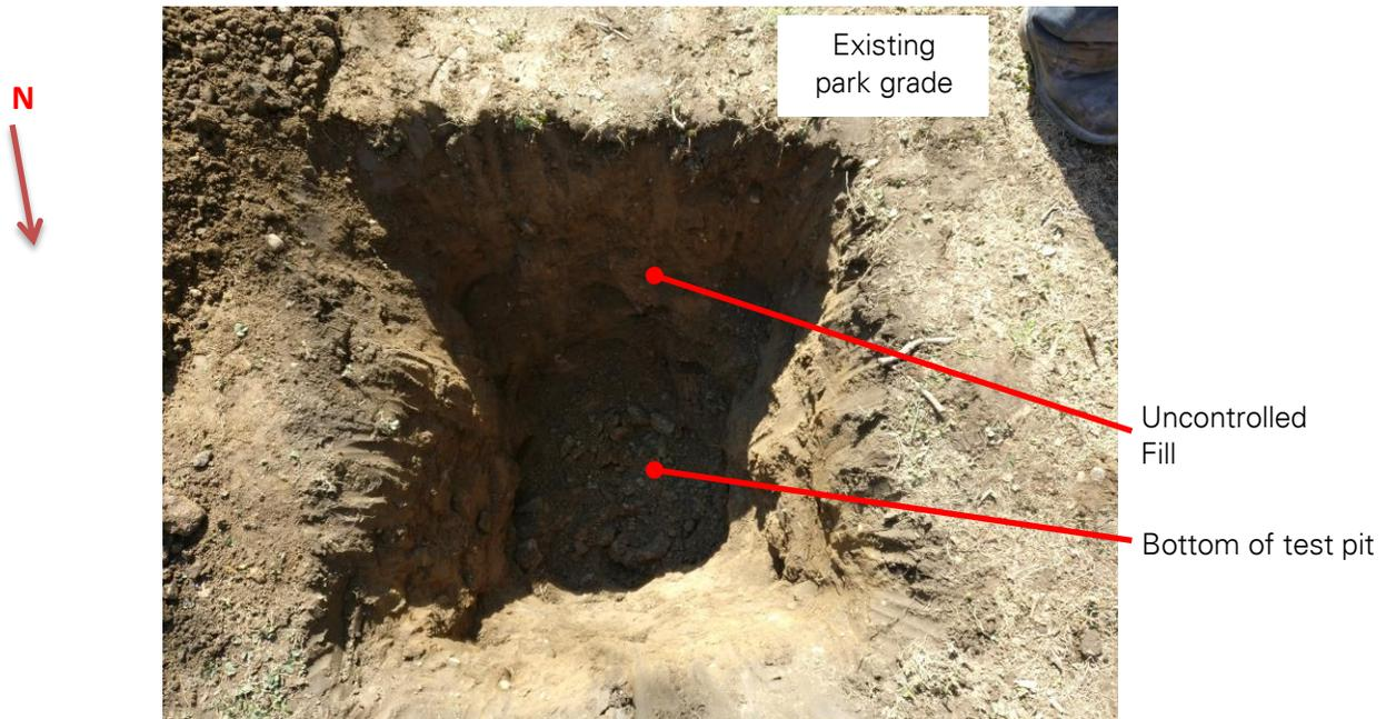
Photo No. 34: LTP-3, General view of the test pit (View: South)
